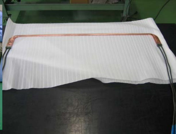
7.5mm conductor (SM2) SUS tube in copper by HIP
