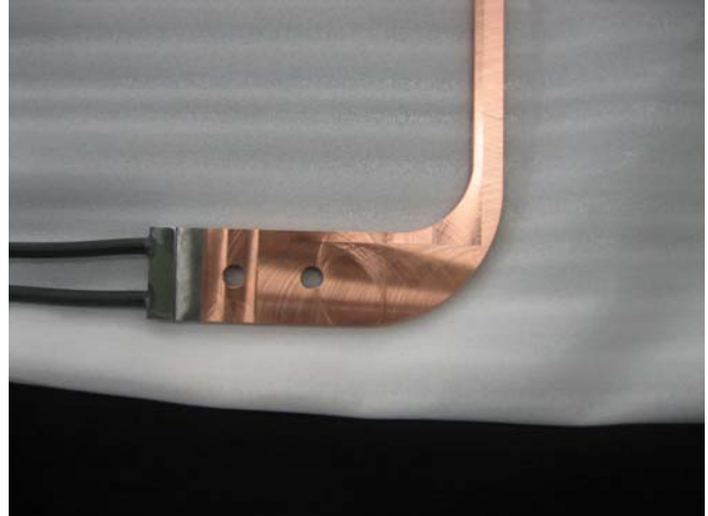
7.5mm conductor (SM2) SUS tube in copper by HIP
