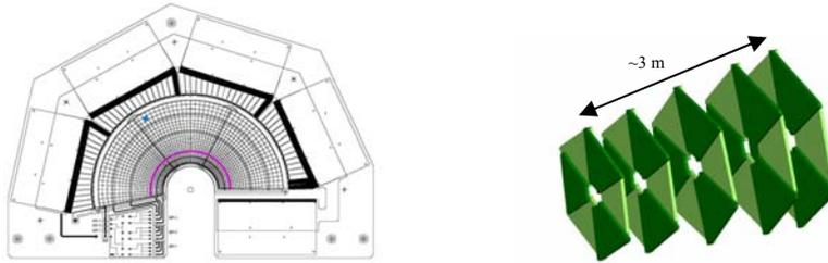
Figure 2. Schematic views of the TOTEM T2 (left) GEM and T1 (right) Cathode Strip Chamber detectors.
