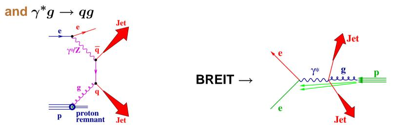
Jets are reconstructed in the Breit frame using a kt-cluster algorithm
