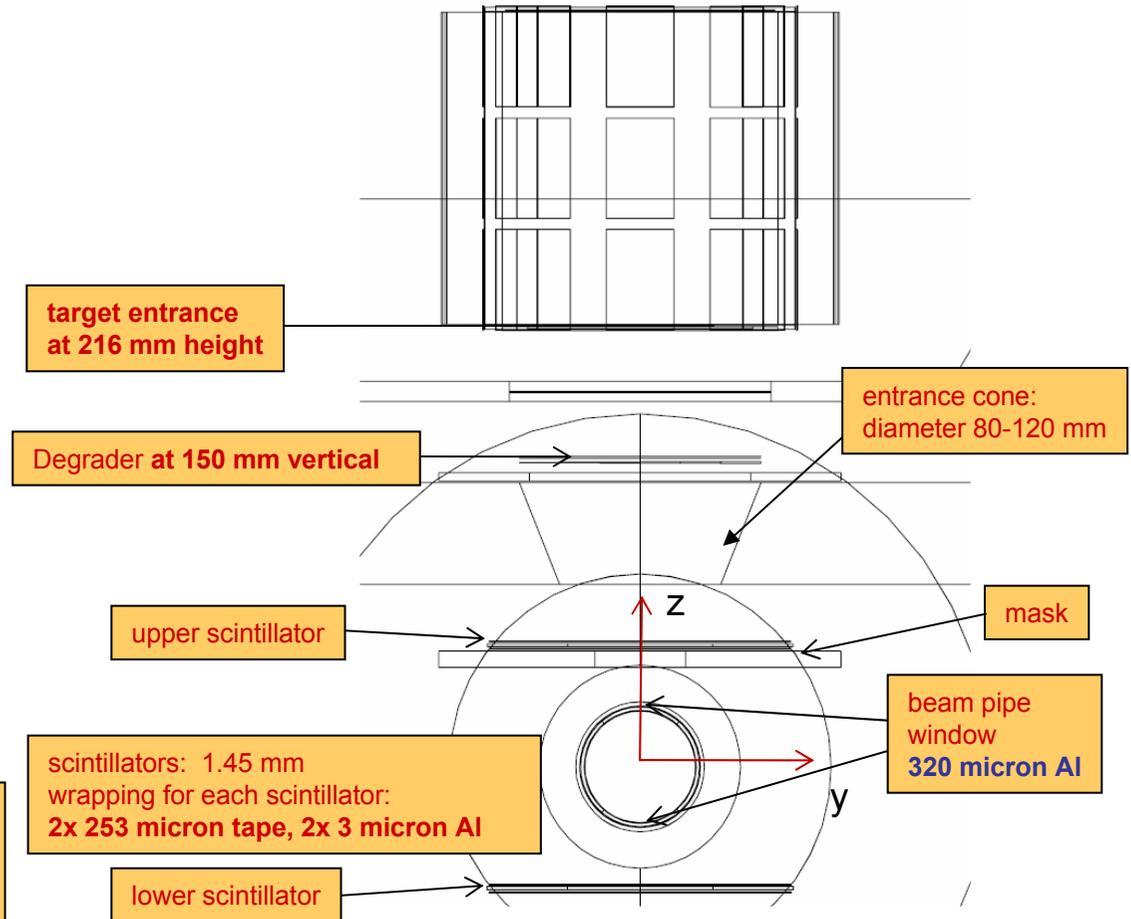
vacuum window: kapton 125 micron + paper 120 micron
