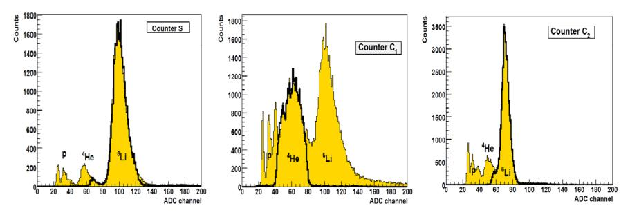
Tuning of trigger counters. Example of signal amplitude spectra obtained for counters of beam monitors S, counters of sets  $C_1$  and  $C_2$  correspondingly. Signal amplitude peaks correspond to lithium beam and its fragments from interactions with target – helium, protons, deuterons. Thick line contours part of spectrum determined by discriminators. Counters S and  $C_2$  are tuned to register lithium, counters  $C_1$  – helium.
