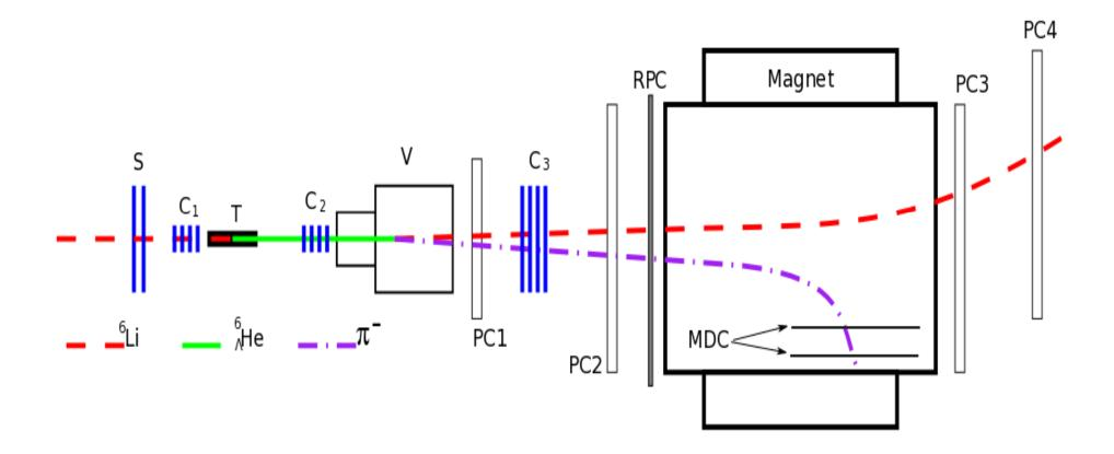
NIS-GIBS spectrometer for  $^6_\Lambda He~$  production with  $^6Li~$  beam. T – target (carbon  $12 \times 3 \times 3~$  cm, 20.4~ g/cm $^2$ ); S,C $_{1,2,3}$  – trigger counters; V – vacuum decay vessel; RPC wall for TOF; M – magnet; PC $_{1-4}$  – proportional chambers, MDC - minidrift chambers (planned in 2011).
