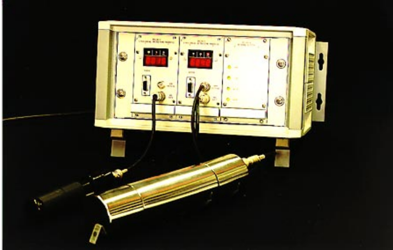
Figure 1. A station crate with two UDMs connected to a Geiger-Mueller tube and a photomultiplier tube
