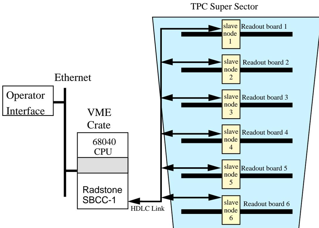
Fig. 2 Hardware configuration for system test. There are six readout boards per super sector, each of which is slave-node daisy-chained by an HDLC cable to a Radstone board. (Each Radstone board can service up to 4 HDLC links, only one is shown.)
