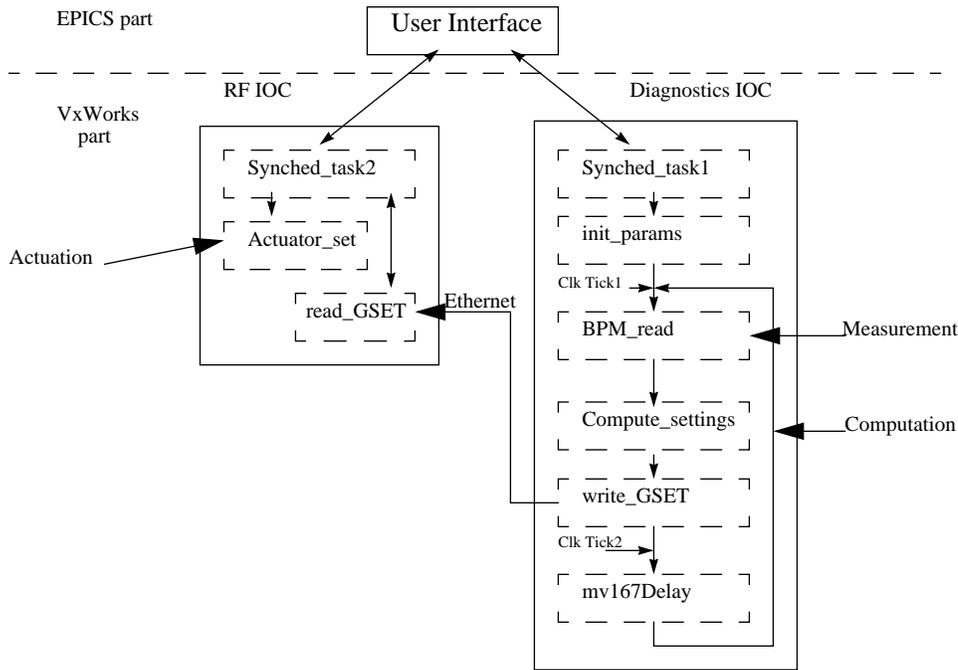
Figure 3: Schematic Software Layout for Energy Lock Loop
