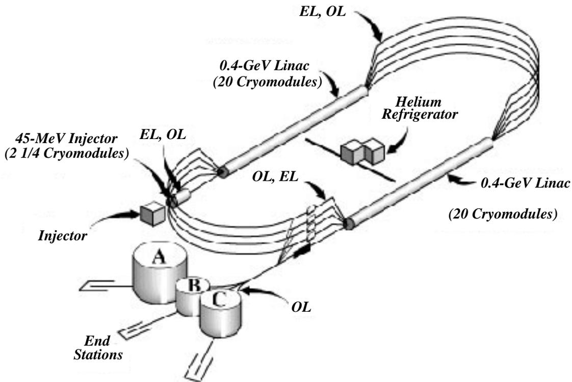
Figure 1: Schematic Diagram with Fast Lock Locations. EL - Energy Lock, OL - Orbit Lock
