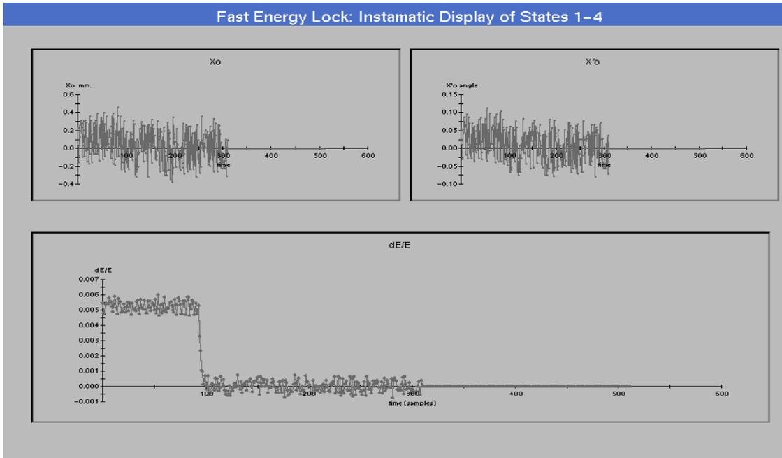
Figure 4: Injector Energy Lock - Effect of closing the loop on  $X$ ,  $X'$ ,  $\Delta E/E$
