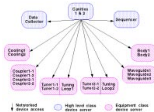
Figure 5. Cavities devices access structure
