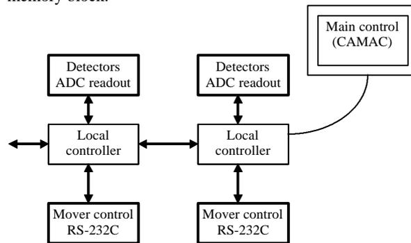
Fig. 4 (Local) control of the Active alignment.
