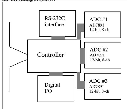
Fig. 3 Hardware level processor functions.
