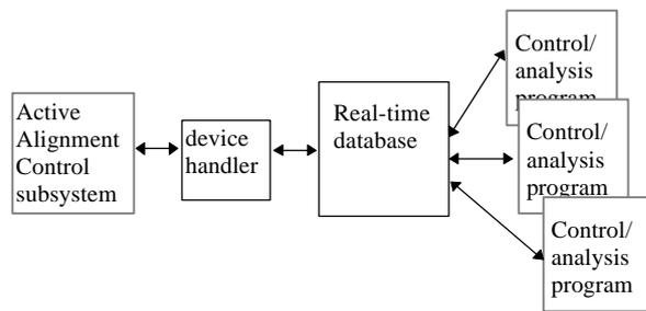
Figure 6. Top level control block diagram
