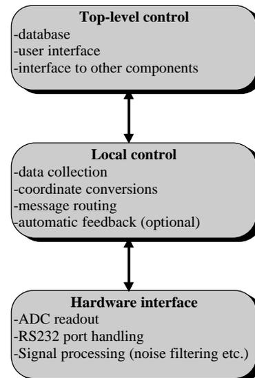
Fig. 1 Control system architecture.
