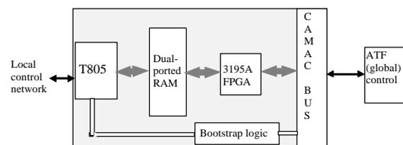
Fig. 5 Block diagram of the CAMAC interface
