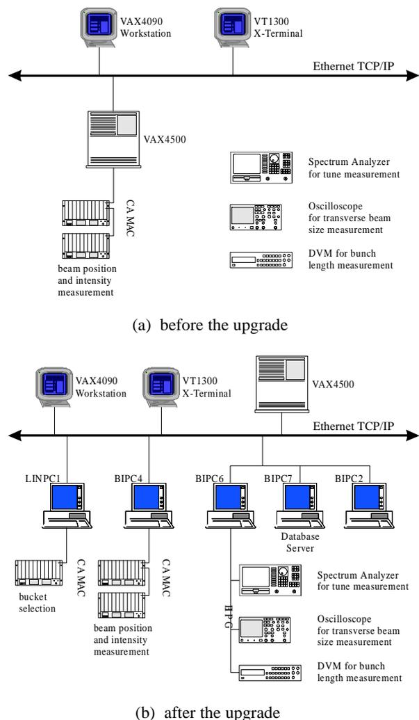
Fig. 1 Schematic block diagram of the BEPC beam diagnostic instrumentation system
