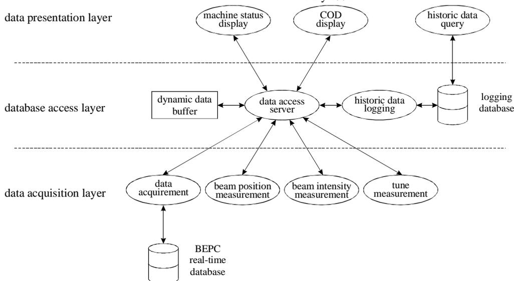
Figure 2: Software structure
