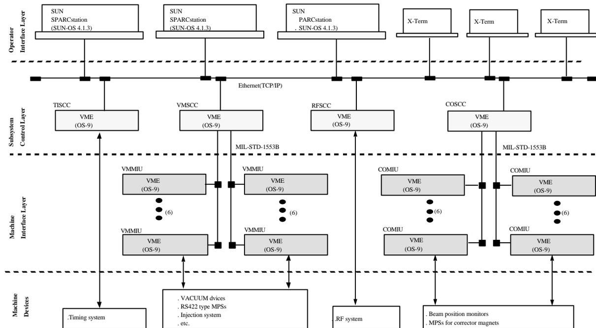
Fig. 1: Schematic diagram of the PLS 2-GeV storage ring control system.
