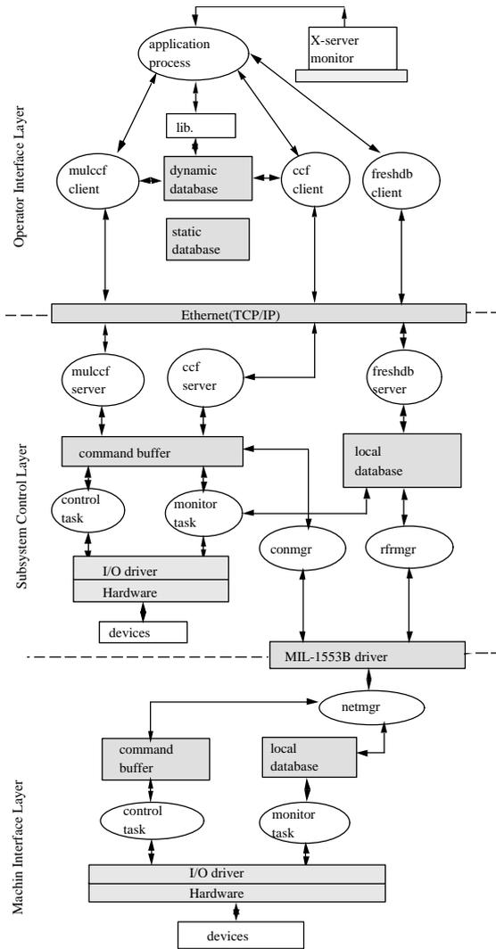
Fig. 2: Software structure of the PLS 2-GeV storage ring control system.
