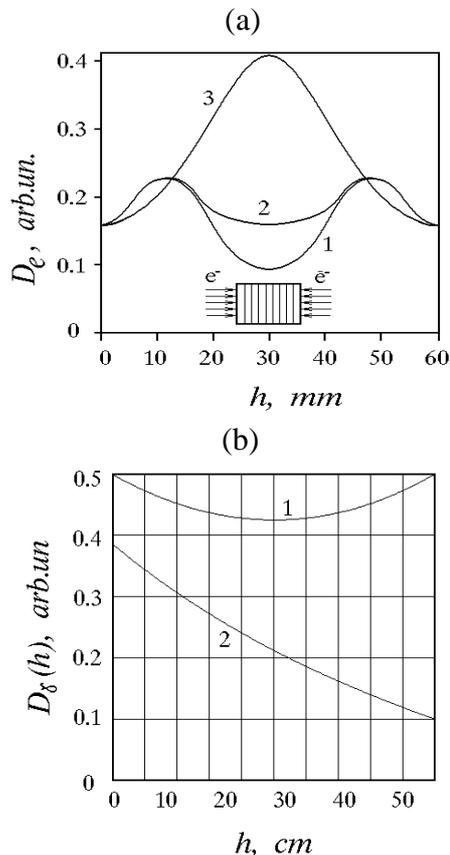
Fig.4 Distribution of electron (a) and bremsstrahlung (b) dose with depth in irradiated compound (wood of aspen + 70 % methylmethacrylate).
