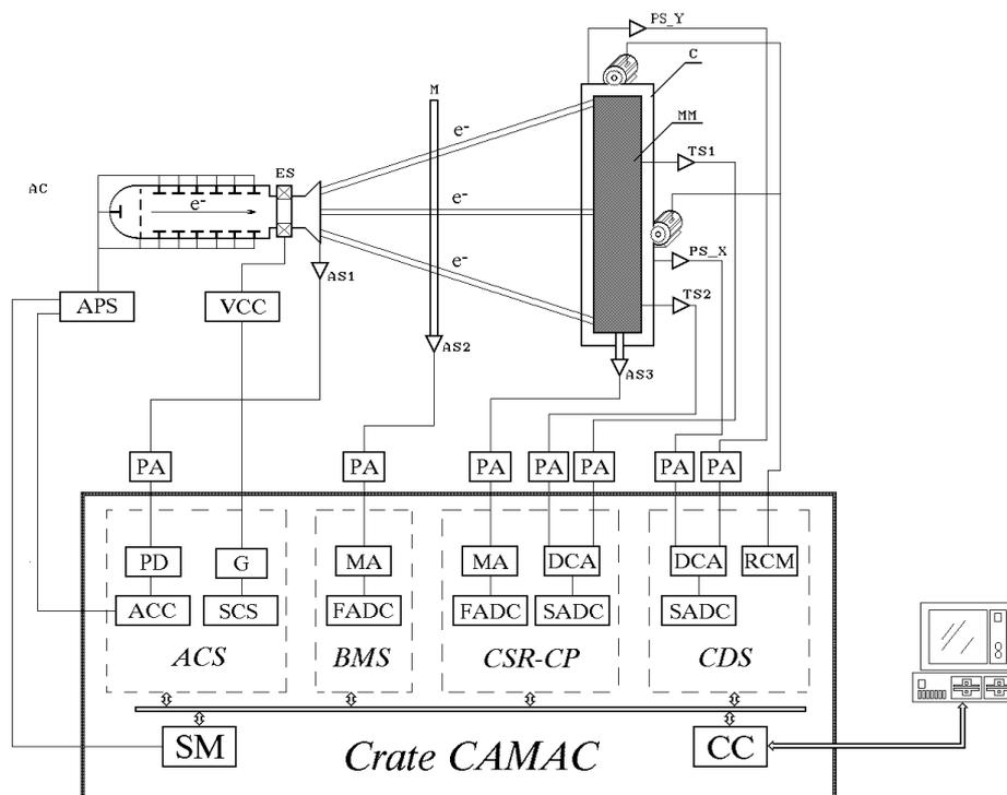
Fig. 2 Block diagram of the radiation facilities for composite materials formation.
