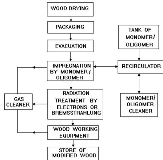
Fig. 1 Technological scheme of polymer-modified wood production.
