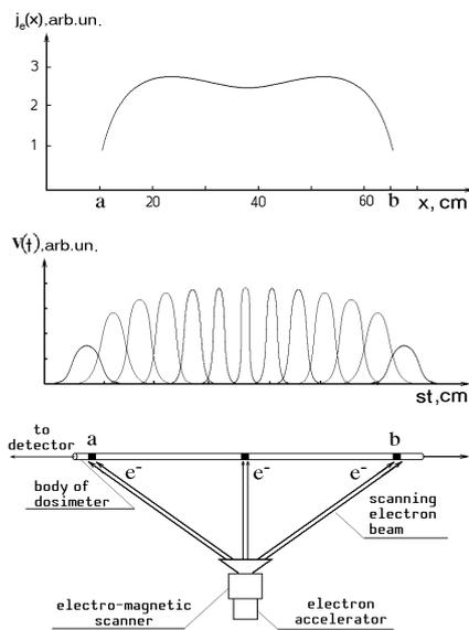
Figure 3. Scheme of utilization of a wire acoustic dosimeter for the monitoring of a scanning electron beam. The current in the scanning magnet had sinusoidal form.
