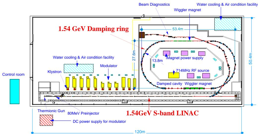
Fig. 1 Layout of the KEK accelerator Test Facility.
