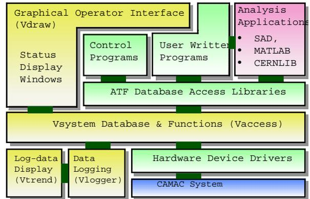
Fig. 3 Software configurations. Vdraw, Vaccess, Vtrend and Vlogger are Vsystem components.
