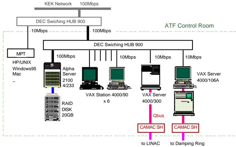
Fig. 2 Cluster configurations in the ATF control system.
