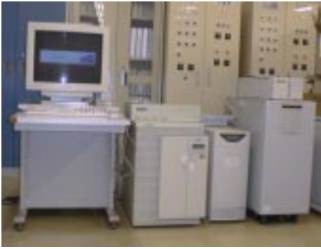
Figure. 4. Mitsubishi ME RK-460 computer running HP-UX 10.20.
