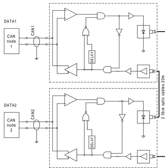
Fig. 3: Fiber-optic CAN interface
