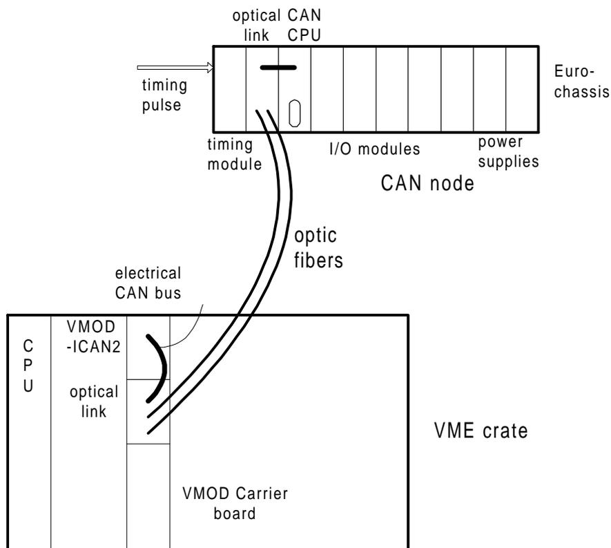
Fig. 2: CAN Net for PS proton source
