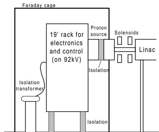
Fig. 1: Proton source for the PS
