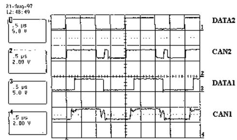
Fig. 4: CAN signals using fiber-optic transmission
