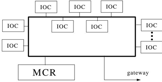
Figure 2 Double ring configuration
