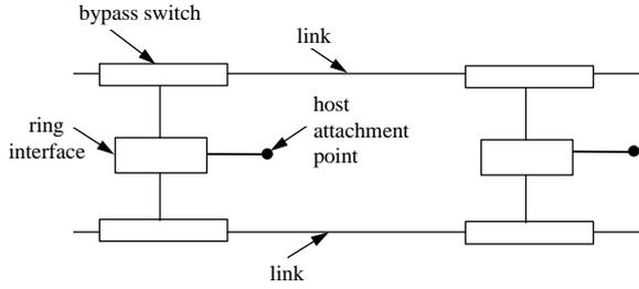
Figure 5 Section of double ring
