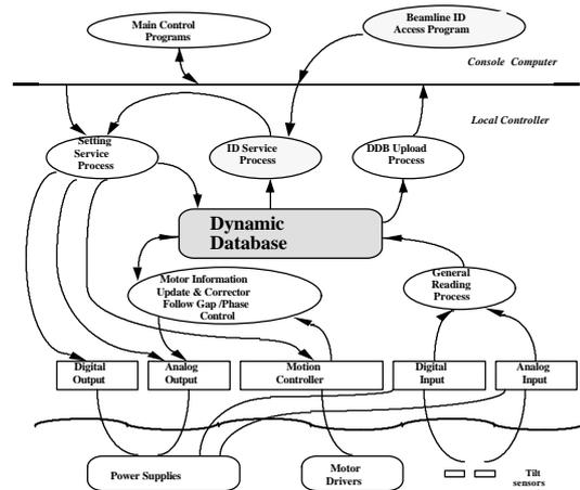
Figure 1. Software structure on EPU controller
