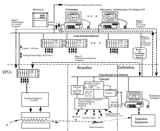
Figure 4. Relation among main control system, EPU controller and the beamline end-station
