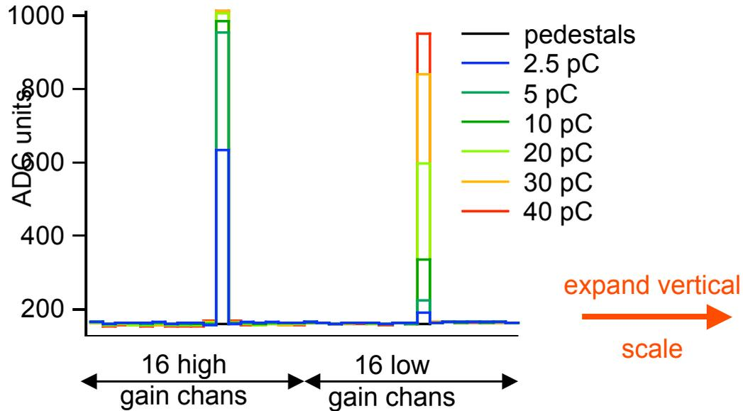
for 500 p.e. signal (40 pC) get ~ 1 p.e. signal in neighbouring high gain channels, and ~1 p.e. depression of pedestals in other high gain channels (~ 0.2 % effects)
