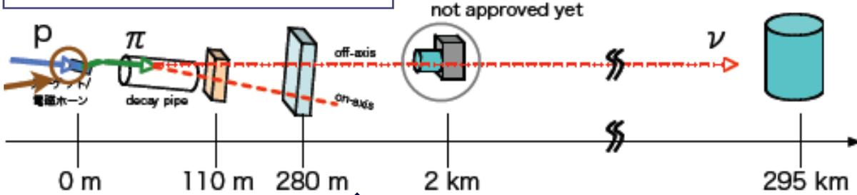
ND280 : off axis beam flux and SuperK backgrounds measurements
