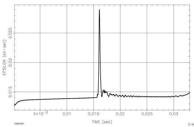
RMS emittance [eVs] vs. time [s] for a high intensity (5 ·  $10^{12}$  protons total) cycle in the Fermilab Booster injector synchrotron with the installed  $\gamma_T$  system operative. The emittance spike near the time of the jump, 15.5 ms, reflects the increase from a few particles soon lost. Note, however, that even the spike is relatively small and the final emittance is hardly changed from the initial.
