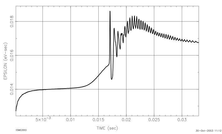
RMS emittance [eVs] vs. time [s] for a high intensity (5 ·  $10^{12}$  protons total) cycle in the Fermilab Booster injector synchrotron with current typical parameters. The irregularity in the later part of the plot reflects particle loss coming from nonlinear single particle effect in addition to the sudden emittance growth caused by NMI.
