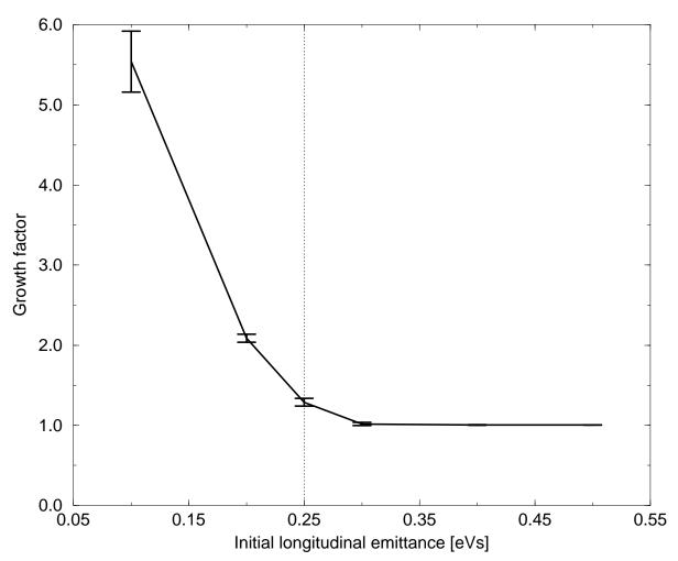
Emittance growth factor vs. initial emittance [eVs] for bunches of  $2 \cdot 10^{11}$  protons crossing transition in the FMI. Each point is determined by a tracking with  $6.4 \cdot 10^8$  macroparticles and a run with  $10^8$ . The statistically weighted mean is the central value with error bars given by the difference between the two runs. The vertical dashed line is the NMI threshold evaluated either from Hardt's perturbation calculation or the self-bunching criterion.
