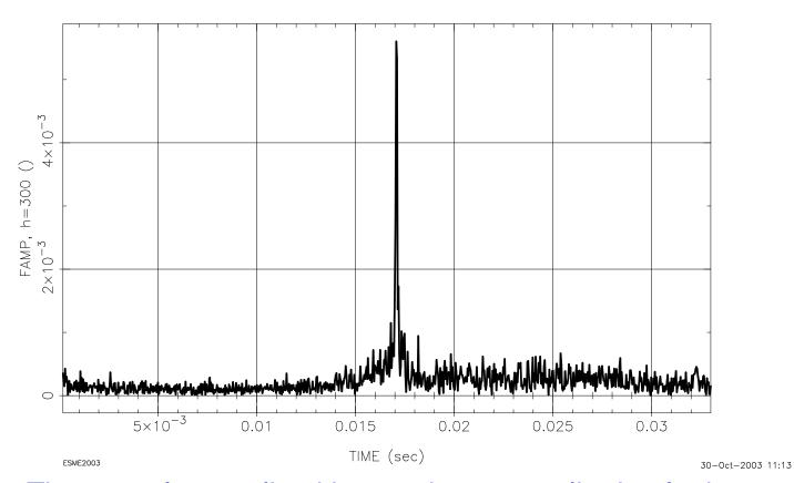
The rms of normalized beam charge amplitudes for harmonics 300 to 319 *vs.* time [s] during Booster acceleration cycle. Note the sudden appearence of these high harmonics just at transition time.
