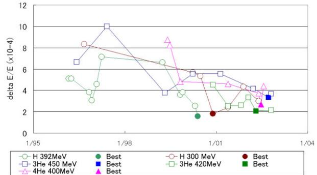
Figure 1. Energy width of Ring Cyclotron Beam
