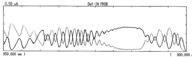
Figure 3. Beam pattern in the outer region measured by deflector entrance probe (thick line: differential probe thin line: integral probe)
