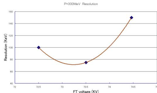
Figure 2. FT voltage and beam energy width (Proton 300 MeV)
