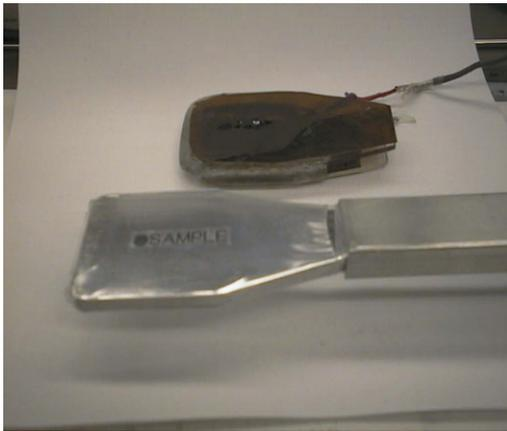
Figure 6. NMR probe head and correcting coil set
