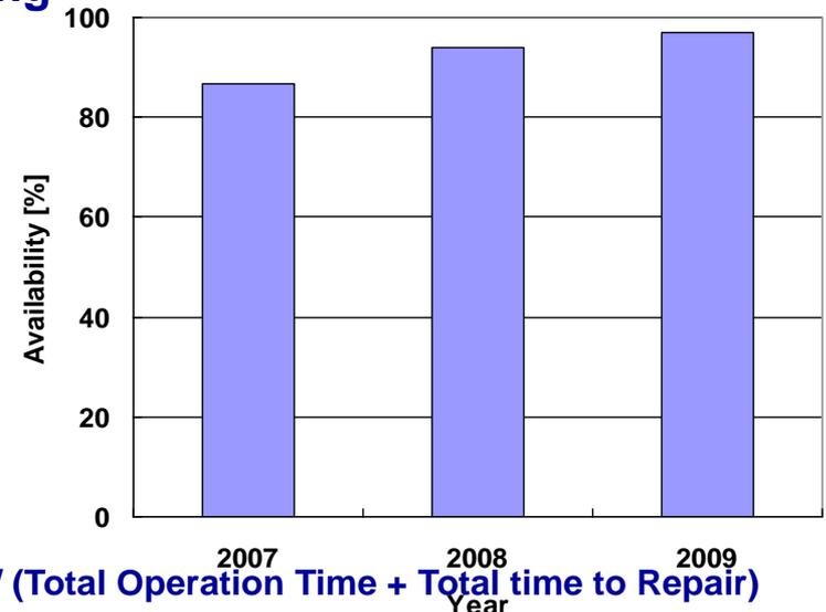
Machine availability = Total Time to Repair / (Total Operation Time + Total time to Repair)
