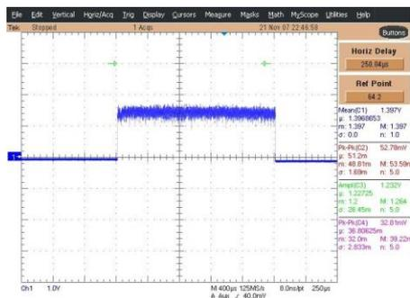
**Long pulse operation (LEBT beam, 2ms pulse)**
