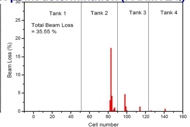
DTL beam transmission (~50%) -> beam loss distribution measurement -> predict the polarity mistake of QM by using PARMILA -> QM polarity reversal -> beam transmission (100%)
