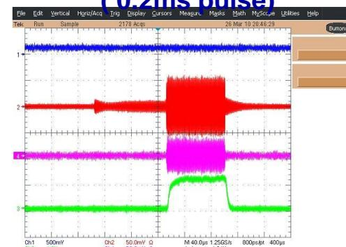
**Beam pulse (DTL beam, 0.1ms pulse)**
