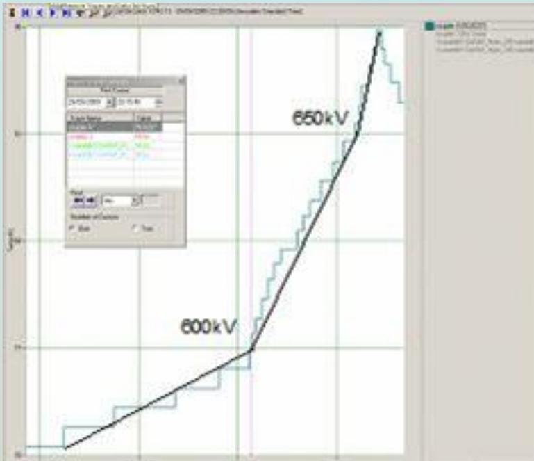
Coupler temperature increase during RF operation in HWR4
