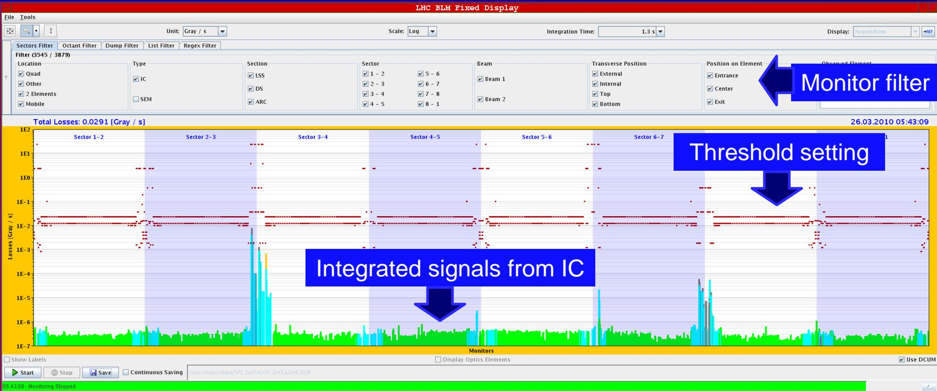
Beam loss monitor readings (Gray/s) along the ring (integration time : 1.3 s)
