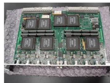
VTR812 Fast ADC Test Board
