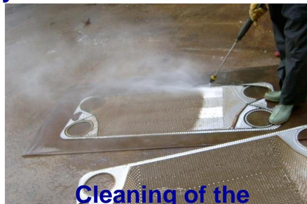
**Cleaning of the heat exchanger plate**
