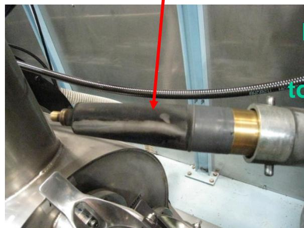
**Change the connector and re-adjust the inside connector (RFQ case)**
