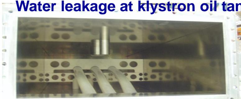
**Leak from the RF load cooling line joint**
