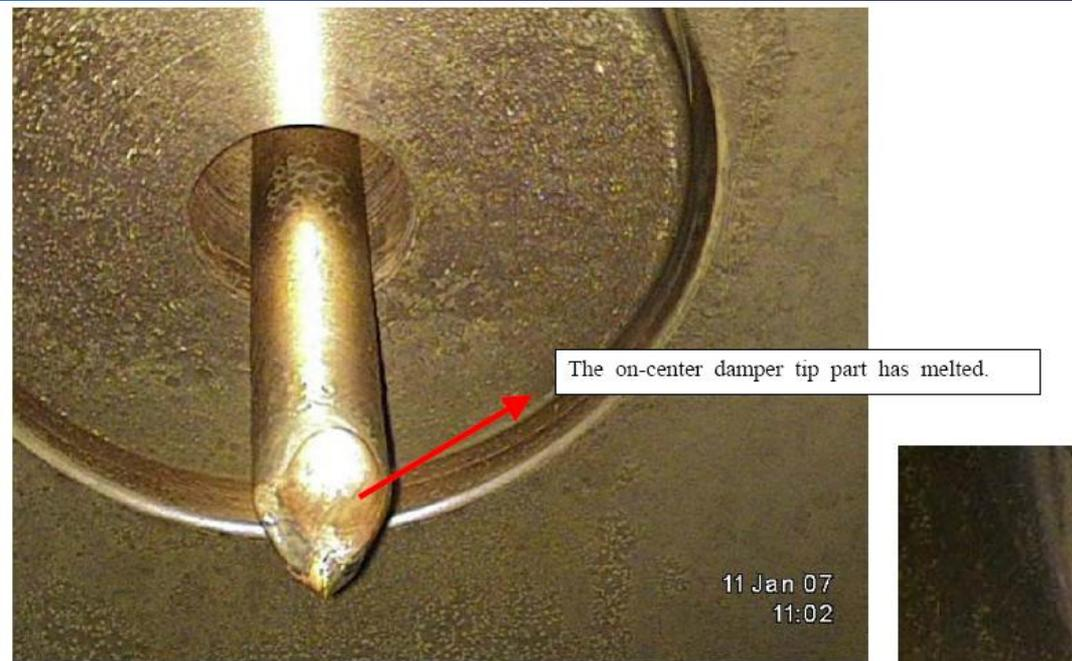
Fig. 2.4 (1) On-center damper copper sheath tip partial photograph
