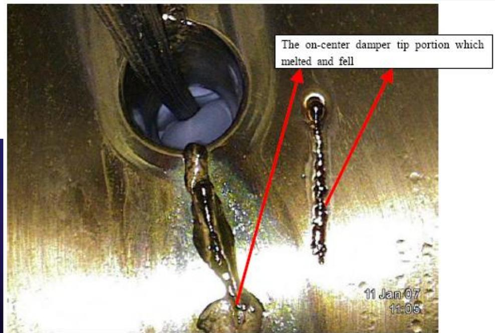
Fig. 2.4 (3) On-center damper tip portion (2) which melted and fell
