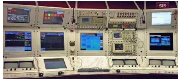
Figure 2: Top: Sketch of the main control room. Bottom: Part of the SIS 18 console with several monitors for operating software, oscilloscopes and a spectrum analyser.
