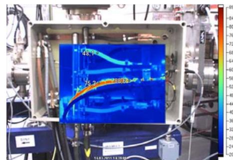
Thermal image of water circuits with persisting plugging (scale max. 89.1 °C).
