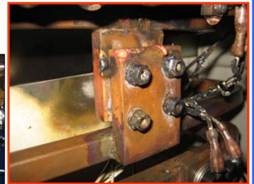
Electrical bridge in the magnet connection box after contact problem.
