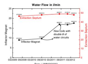
Water flows of magnets with 35 °C temperature rise (in/out) since 2009.
