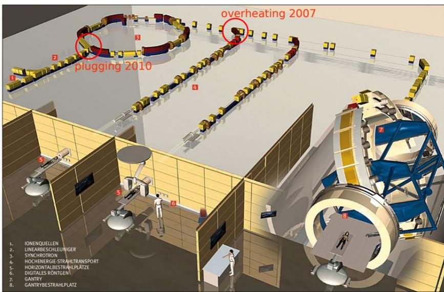
The Heidelberg Ion Beam Therapy Centre with 1. ion sources, 2. linear accelerator, 3. synchrotron, 4. high energy beam transport line, 5. horizontal treatment rooms, 6. digital x-ray imaging, 7. gantry, 8. gantry treatment room.
