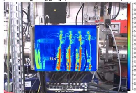
Thermal image of the water circuits after repair (scale max. 40.4 °C).
