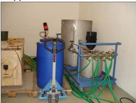
Passivation device from GSI Darmstadt connected to a spare coil.
