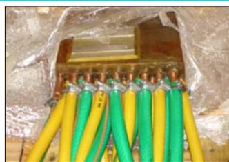
Water hoses connected to the spare coil of the extraction septum.
