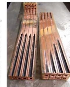
Copper oxide (CuO) layer inside the cooling channel of the inflector magnet.
