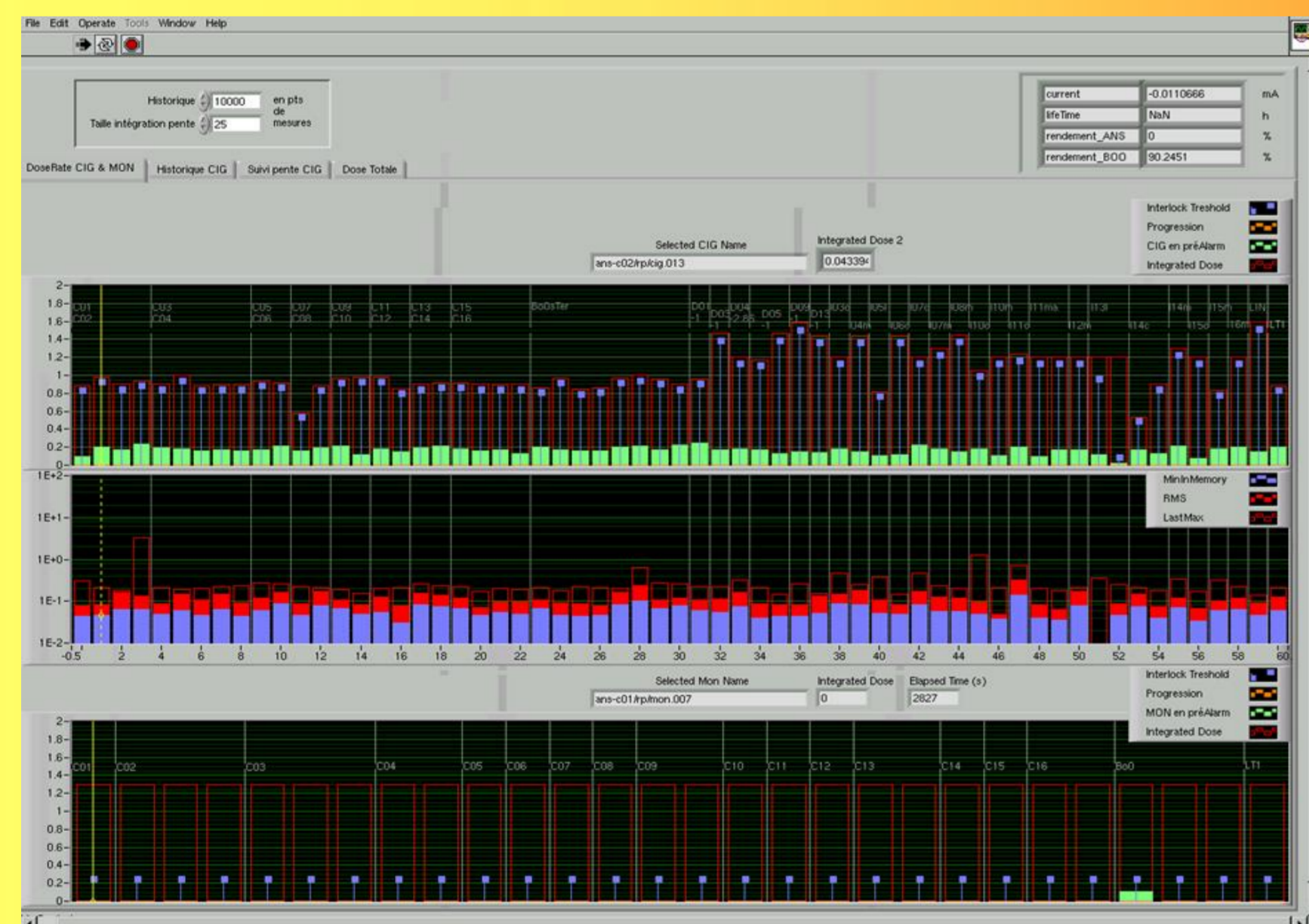
Monitoring of gamma ionization chambers to rapidly detect any anomaly and avoid, if it is possible, interlocks
