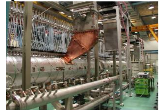
20MeV DTL 4 Tank 150 Drift tube Electroplated Tank Pool type Electromagnet
