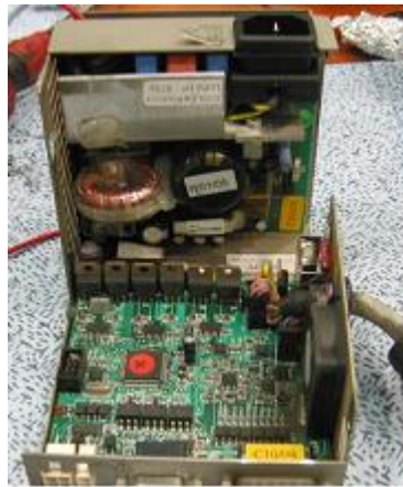
TMP pump controller
