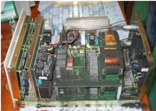
Ion pump controller
