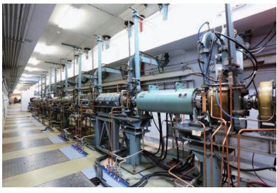
60 MeV electron linac. The Great East Japan Earthquake caused serious damage on the accelerator facility in ELPH. Only low energy part of 300 MeV linac was salvaged refining high voltage pulse unit for Gun and the components of the transport section.
