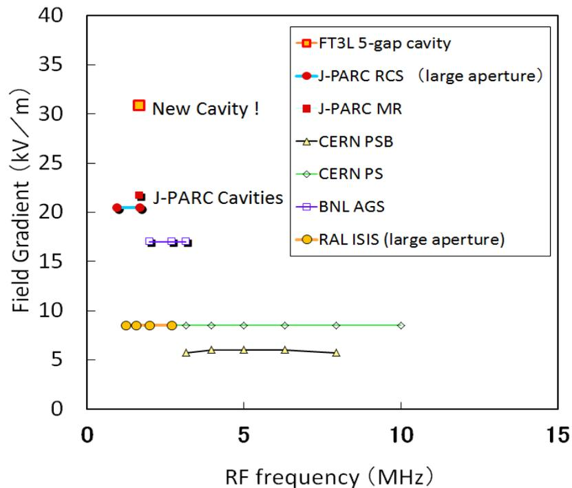
Performance of cavities depends on core materials: ferrite and MA.
