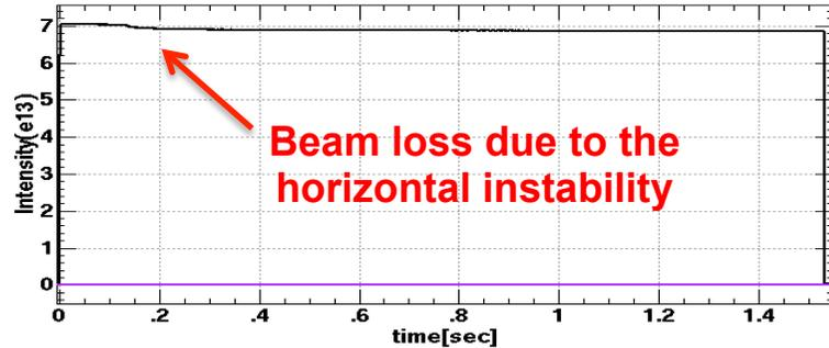
Extracted beam : 6.82e13 ppp (132 kW eq.)
