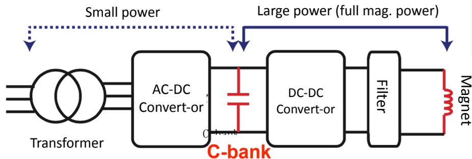
Two large converters and large capacitance for energy recovery, symmetric power module circuit
