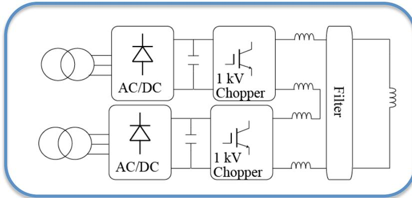
Diode rectifiers, two 1kV choppers are connected in series, symmetric power module circuit
